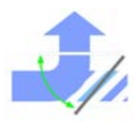
3-WAY DIVERTER DAMPERS For changing over gas flow or simultaneously isolating one duct.
