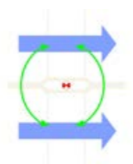
BUTTERFLY DAMPERS Typically installs to isolate & control flue gases
